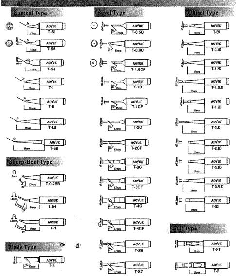
Suitable for all ACYUE soldering irons except lead free composite tip series, induction series and 938
